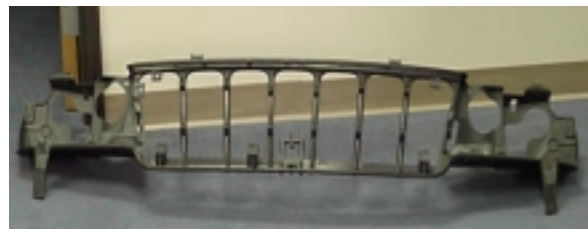
Figure 5: Gas-Assist Reduces the Number of Gates
